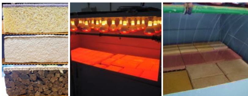
On the left: ETICS solutions; at the centre: Uv-IR irradiation aging tests; on the right: freeze-thaw cycles artificial aging tests
